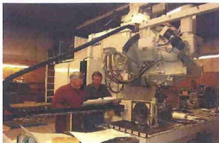
Solar Lens Manufacturing: Our mold-making machine was delivered in 2008. This machine takes 3 months to etch the thousands of intricate grooves into our lens molds.
