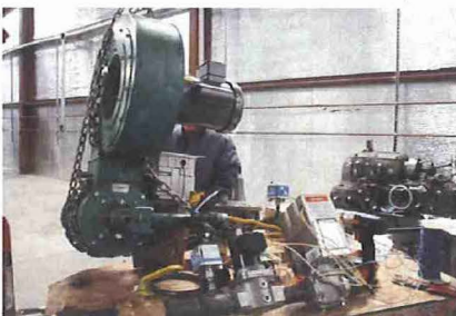
Early Manufacturing: The turbines are designed to run off of solar heat and any other heat source. Shown is a biomass burner.
