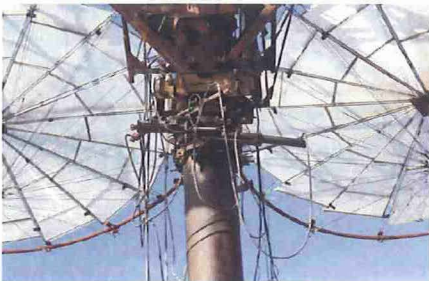
Prototyping: Early prototype of the hydraulic dual-axis tracking system.
