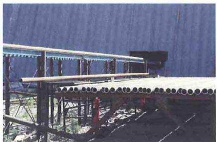
Manufacturing: The automated system for feeding cut pipe to the pipe bender. They red rams underneath lift the pipes up to the feed system.
