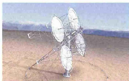
Four-Disc Concept: After successfully proving the tower concept many configuration designs were considered. The four-disc designed was adopted because it gave the greatest cost and assembly advantage.
